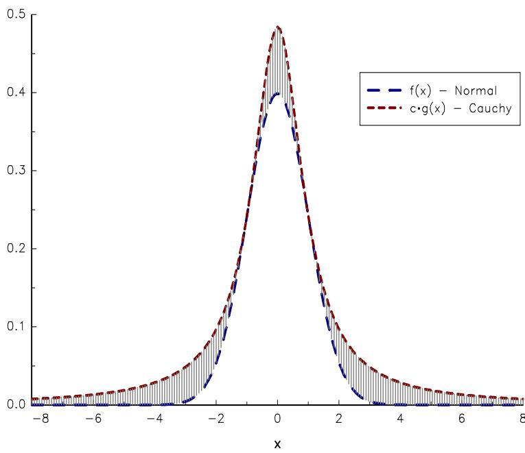
**FIGURE 13.3:** Rejection sampling applied to the normal distribution
