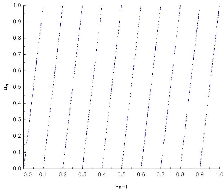
**FIGURE 13.1:** Lattice structure of the linear congruential generator
